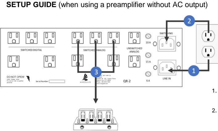
Alternatively, if using a preamplifier without an AC outlet or an integrated amplifier, connect a power cable from one of the QR-2's Unswitched outputs to the Switching Input. Then connect your preamplifier or integrated amplifier to one of the Switched Analog outputs
